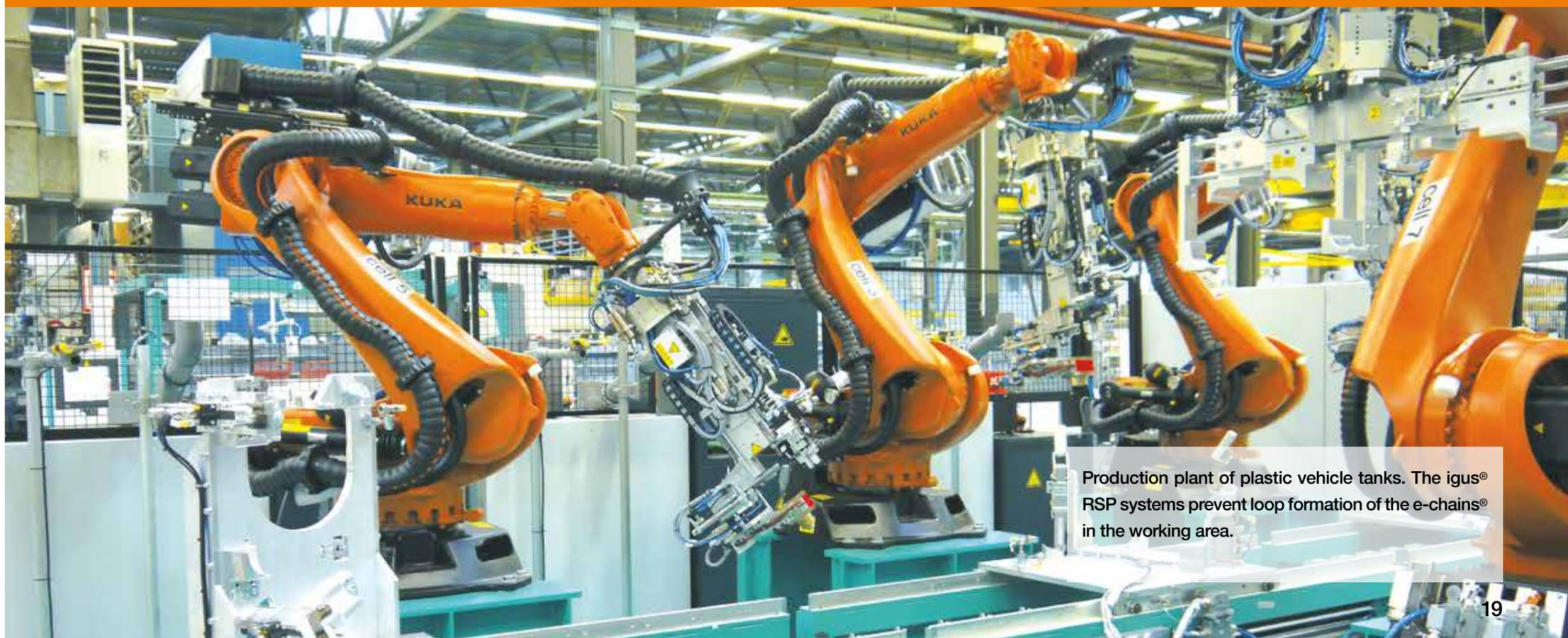
Production plant of plastic vehicle tanks. The igus® RSP systems prevent loop formation of the e-chains® in the working area.
