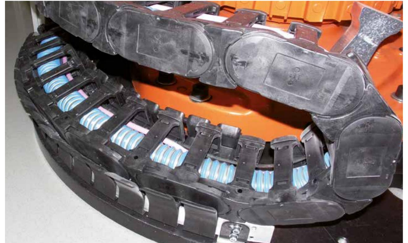
twisterchain application on a cleaning robot
