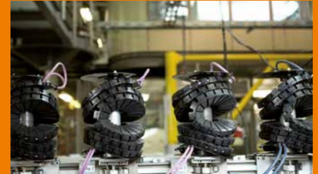
Test for torsion and twisting
