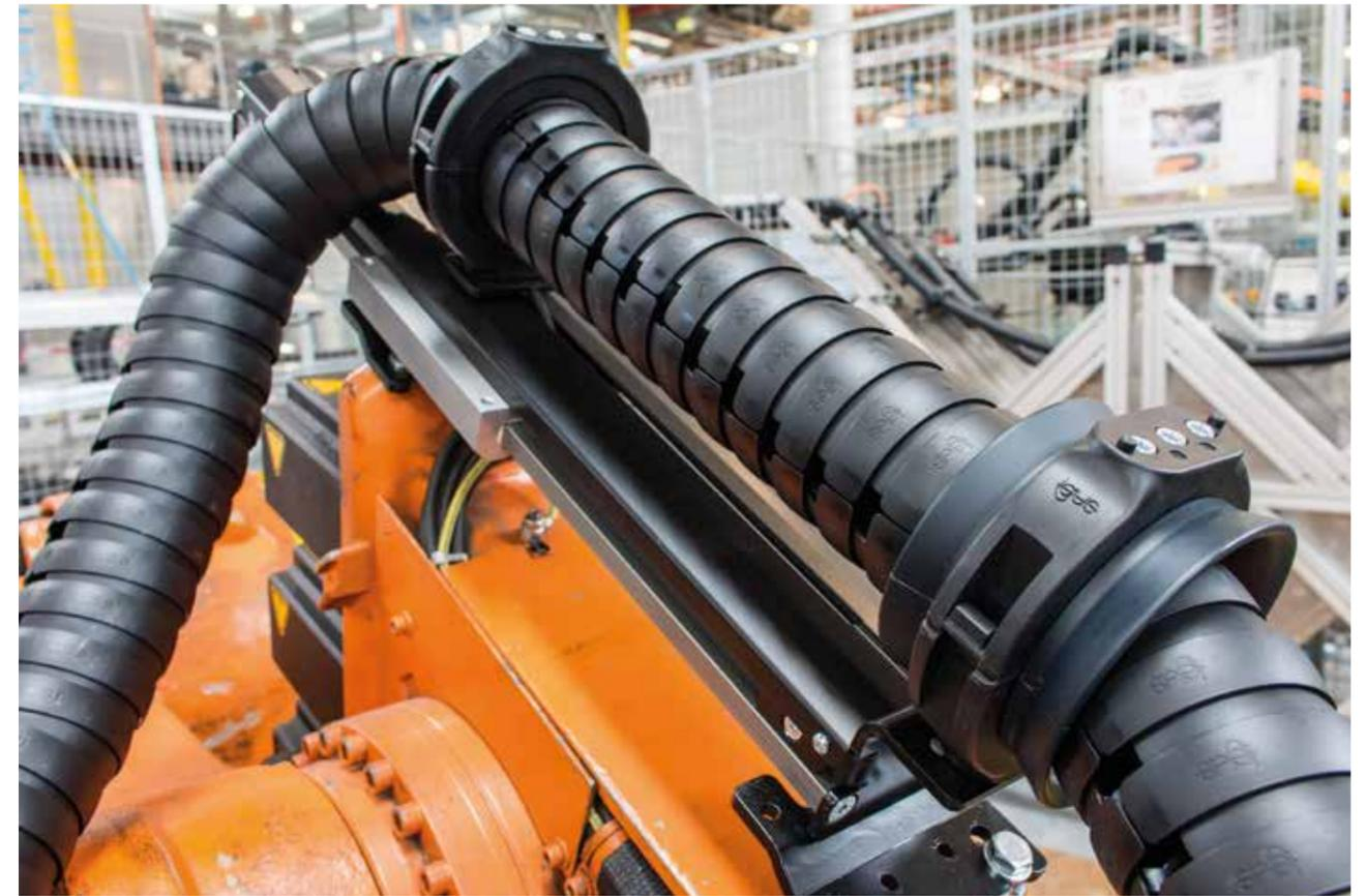
igus® TR.RSE system on test robot
