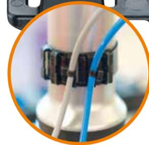
Single cables and hoses are attached with cable tie-wrap
