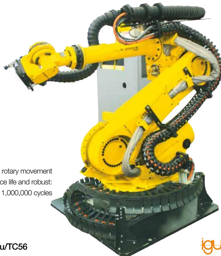
twisterchain in a guide trough for rotary movement on an articulated robot - long service life and robust: tested successfully for more than 1,000,000 cycles
