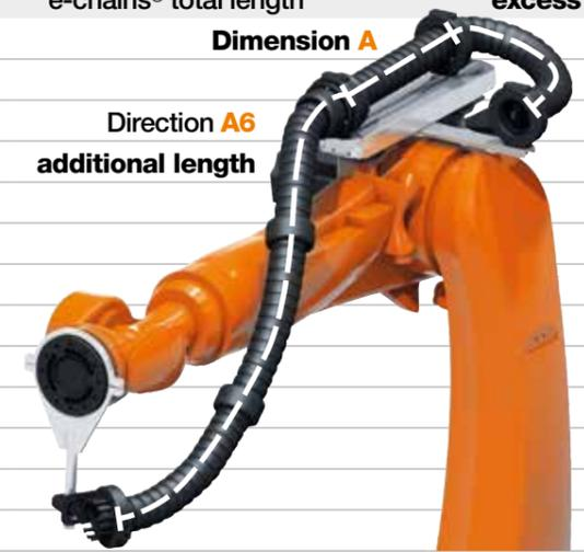
To calculate the e-chain® total length: please add the additional length A1, the additional length A6 and the dimension A. Additionally, at least 1 limit protector must be ordered
